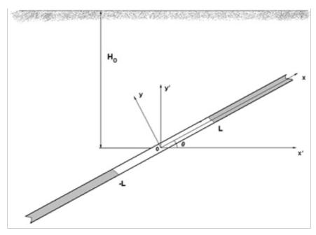
**Figure 1 -** Schematic representation of an inclined formation and coordinate systems used
