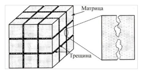
Figure 4 - Conceptual block model of the structure of coal
