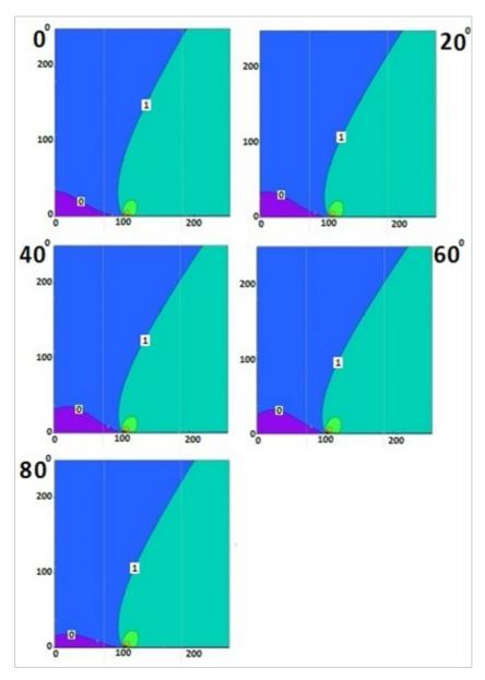
**Figure 3 -** Unloading zones in the roof of an inclined formation (formation angles are indicated)
